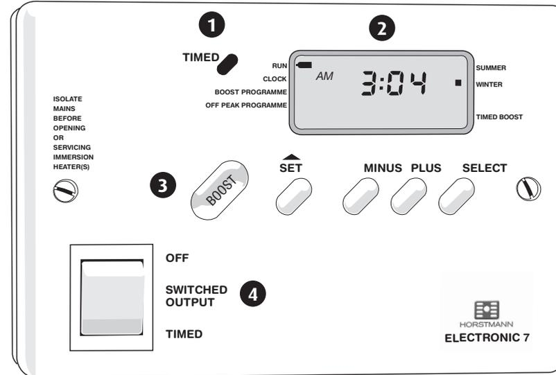
LCD Display: The LCD display allows the user to view the current time and set programme times.
