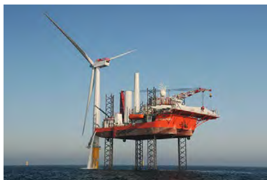
Figure 2.6 Example Construction Vessel (Jackup Barge)
