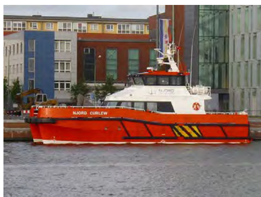
Figure 2.7 Example Crew Transfer Vessel (fast, often multi-hull vessels)
