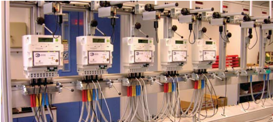
Automatic meters undergoing rigorous testing before installation.
